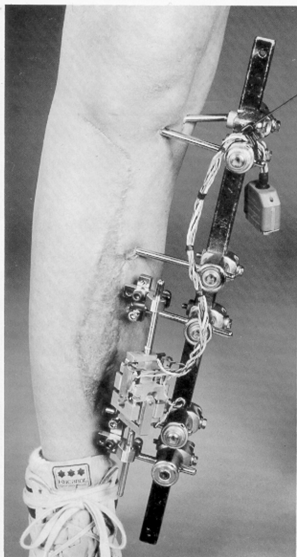
Figure 1. The Oxford Micromovement Transducer (OMT) attached to the bone screws of an external fixator. Dynamic interfragmentary displacement is monitored continuously in six degrees of freedom at the centre of a tibial fracture site.
